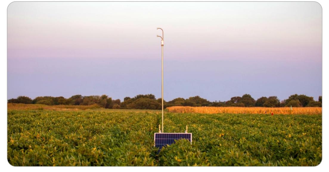
LI-710 is a simple-to-use device which directly measures ET, sensible heat, temperature, humidity, and atmospheric pressure every 30 min.
